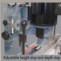
Adjustable height stop and depth stop
